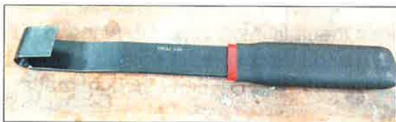
Pictured is Finn’s manufactured spot weld chisel.
