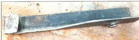
Here is the tool Matt originally invented out of an old bed frame section.
